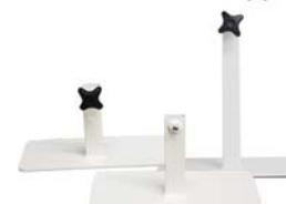
**⚠ NOTE! A safety limit marking (hole) is marked on the lower edge of the upper support (5cm). The upper support must be installed in such a way that the marking is not visible above the floor support.**
